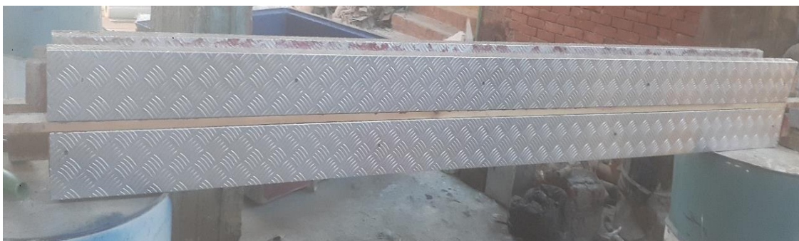
Fig. 5: The aluminum chequered plate mould used for manufacturing of FRP forms.
