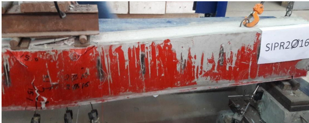
Fig.17: Failure mode of the specimens with FRP SIP forms, the second mode.
