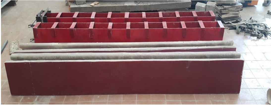
Fig. 6: The FRP forms used for stay-in-place RC beams.
