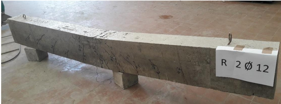
Fig.16: Failure mode of specimen (R 2Ø12), the first mode.
